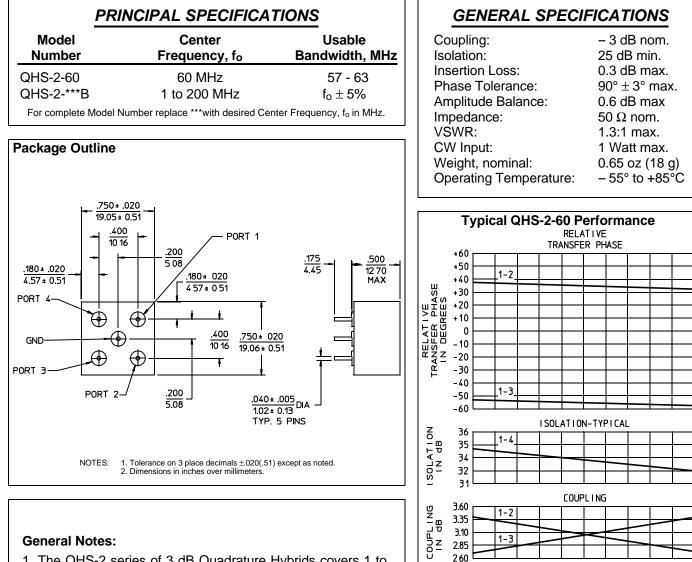
1. The QHS-2 series of 3 dB Quadrature Hybrids covers 1 to 200 MHz using a special lumped element design to reduce the size making it ideal for applications where high performance and PC packaging are required.
